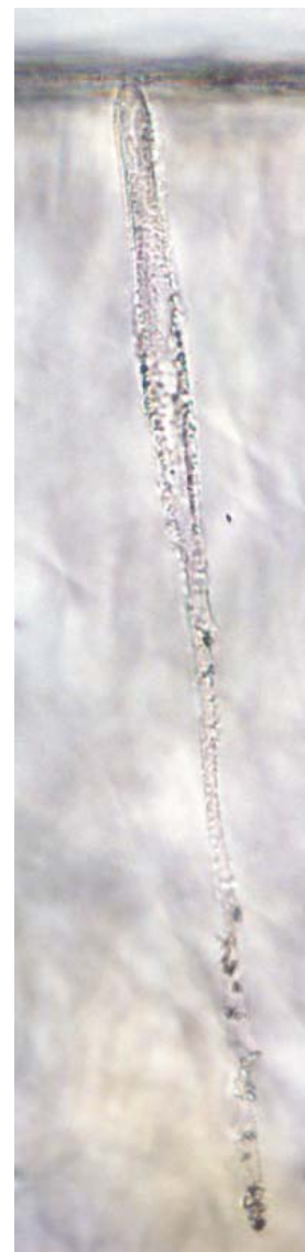
Fig. 2. A millimeter-long track of a Wild 2 particle in aerogel. The particle entered at the wide end. The force of impact broke up the particle; consequently, each black dot is a small cometary rock. [Image: JPL]
